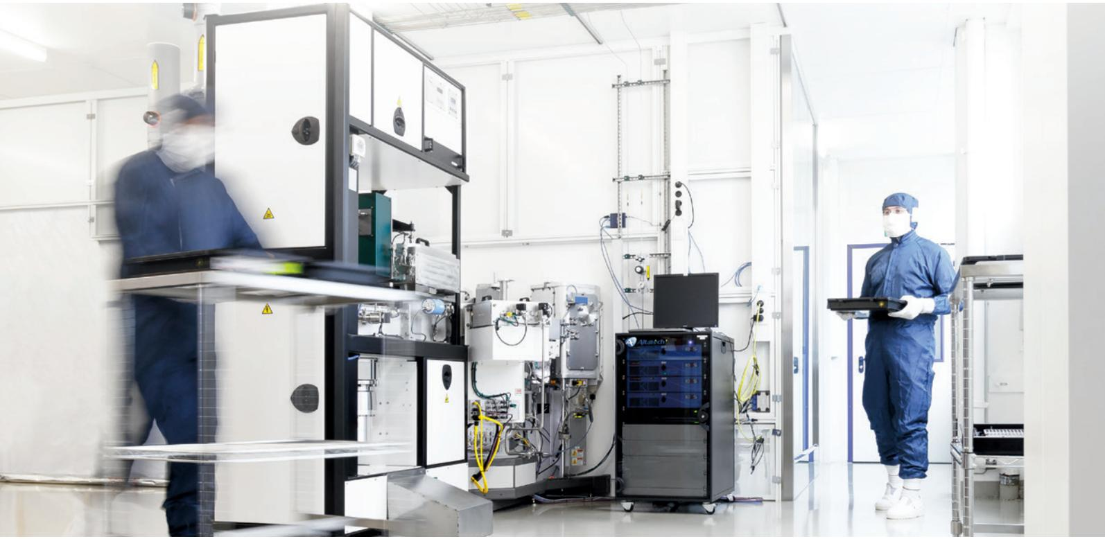
In order to comply with the High Purity and Ultra High Purity (UHP) requirements of the semiconductor industry, WIKA UHP and HP products are cleaned, packaged and preserved in accordance with SEMI specifications. All UHP products are 100% helium leak tested to  $1 \times 10^{-9}$  scc/sec (inboard) in an ISO class 6 cleanroom or better.
