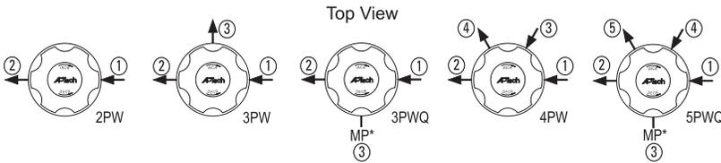
MP=Monitor port, first stage outlet pressure (second stage inlet pressure). Number at each port note order for specifying fitting type.
